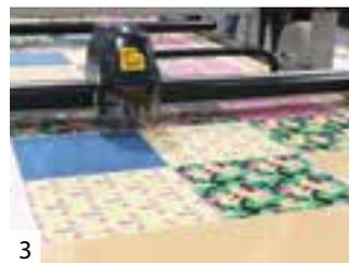
3 Gerber Z1 single-ply cutter with ContourVision cuts fabric panels
