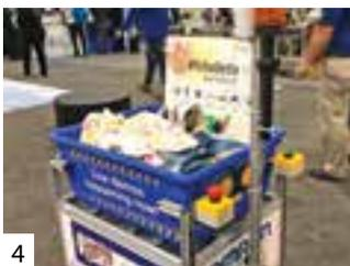
4 'Gerbie' Omron robot powered by Henderson Sewing Machine transports cut panels to sewing section
